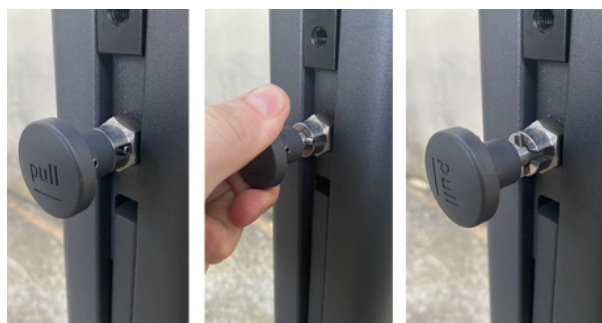
12 (above) - The process of unlocking the rotation button. Notice the 'arms' of the button come out of the groove and rest on the perimeter.
