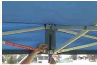
10. Secure internal velcro tabs to keep canopy taut over the frame.
